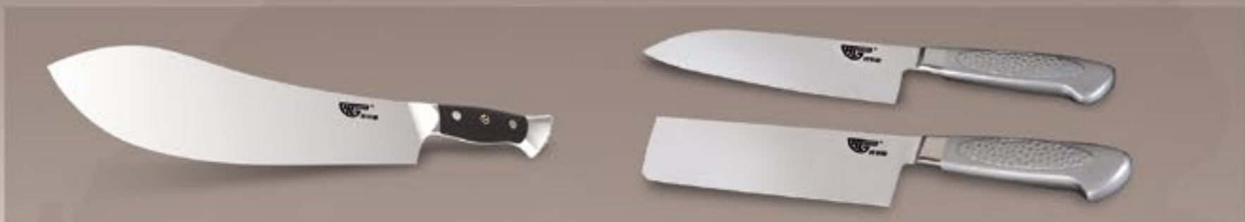
Chef's knife with unique design (DK-4002) • Ice-hardened X50CrMoV15 steel blade from Germany; 55-57HRC • 10-11° edge angle • 7-8N cutting force
