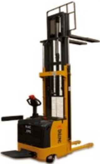
Electric pallet stacker, 1,200-2,000kg rated load
