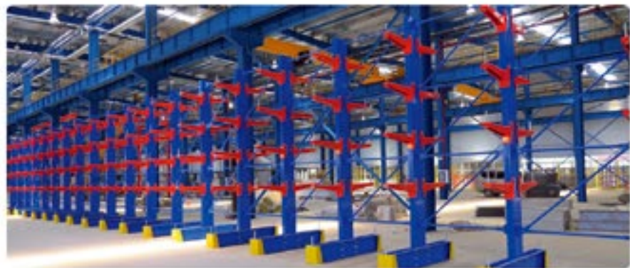
Cantilever racking
