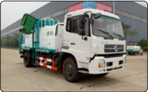
Waste disposal truck, used for collecting and transporting household garbage, food waste and urban sludge
