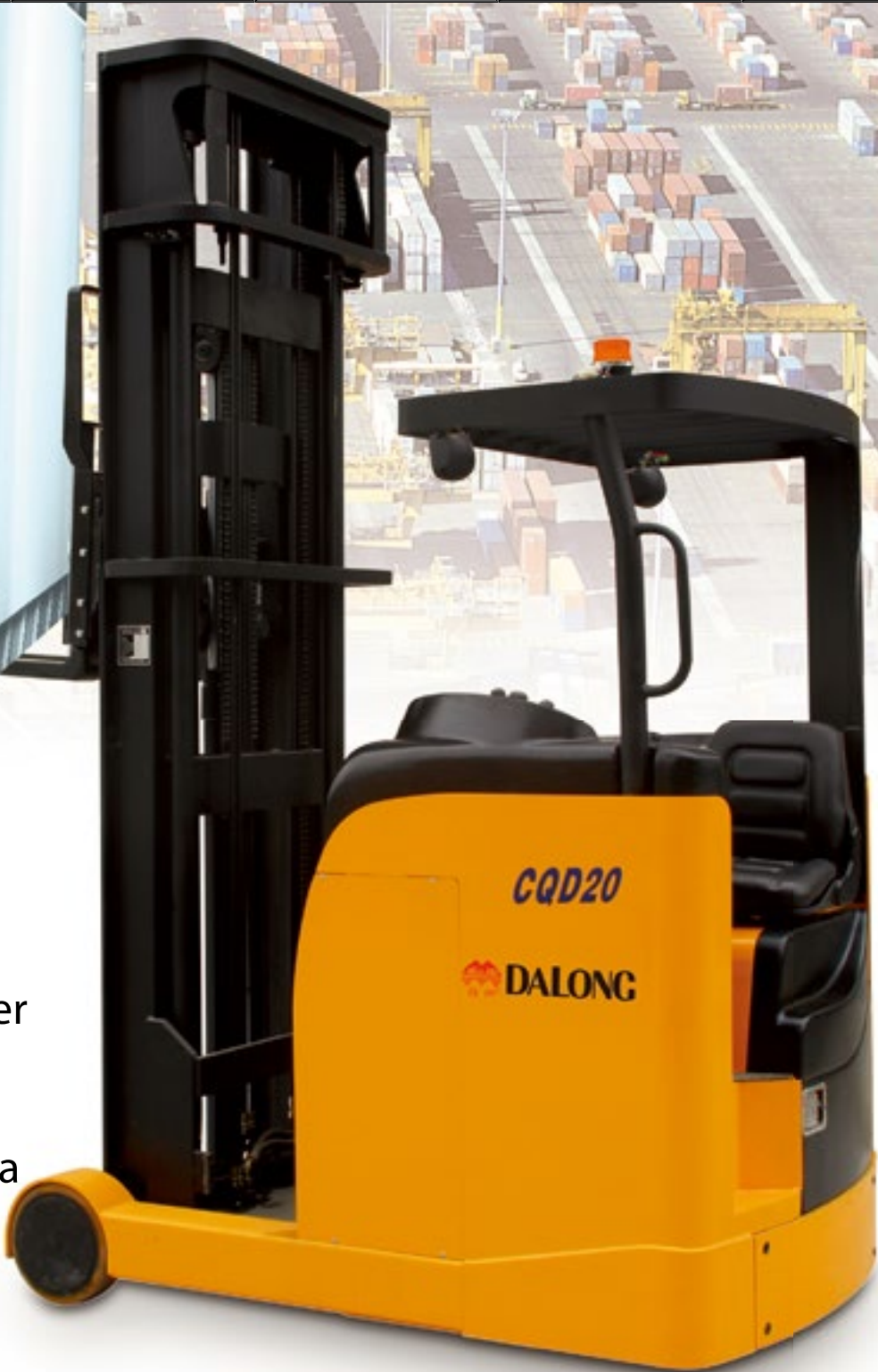
Electric reach truck, 1,500-2,000kg rated load
