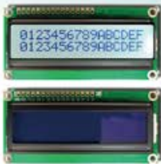
MTB1602A • Display character: 16 x 2 • Display color: STN/FSTN • Mode: positive, negative, transmissive and gray
