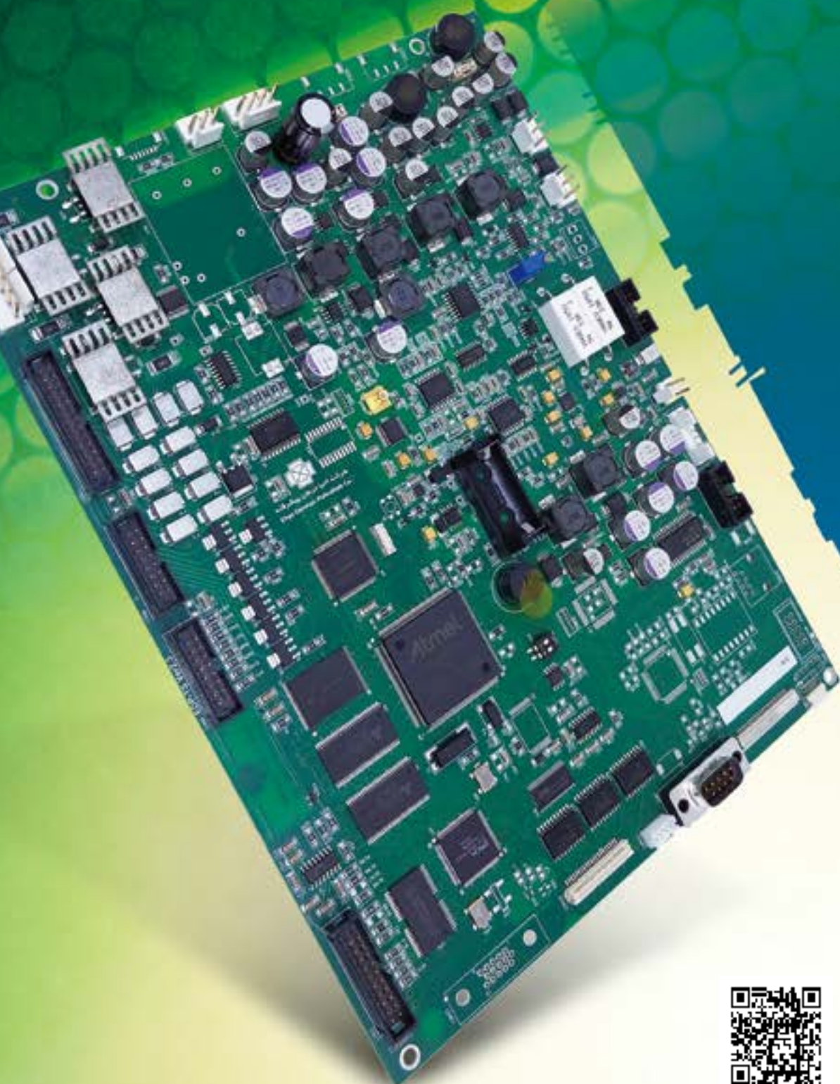
8-layer PCBA with impedance control for industrial equipment
