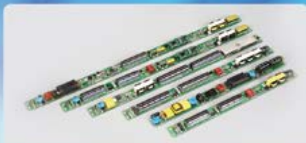
9-70W LED drivers for T5/T8 tubes
