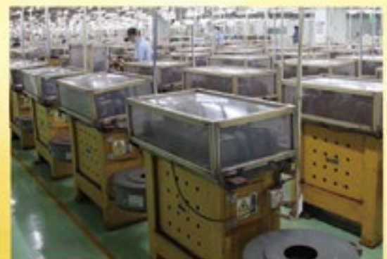
Dumet and CCS assembly machines for glass-molded packages
