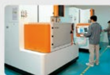
Slow-feed wire cutting machine
