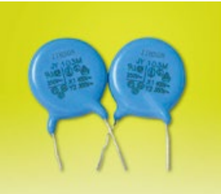
Jimson's model CT8Y2 ceramic capacitor has 10 to 10,000pF measured at 1kHz±10 percent, 1 to 5V rms and 25 C.
