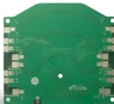
4-layer high-frequency immersion tin PCB
