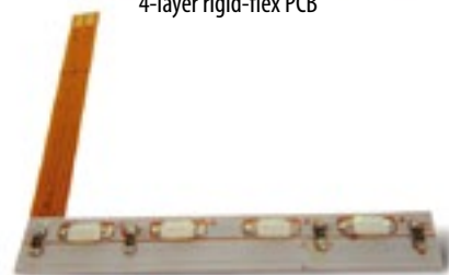
Double-sided flexible PCB, for backlight solutions
