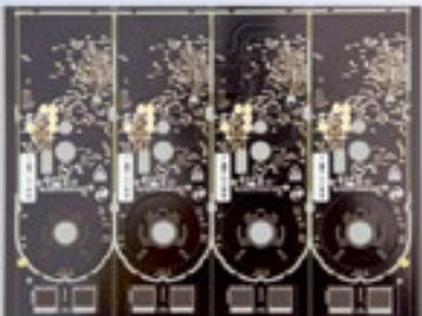
4-layer PCB with ENIG and carbon printing
