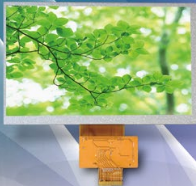
5" color TFT LCD module • 800 x 480 resolution • 24-bit RGB interface • Brightness: 320 cd/m 2 • Optional capacitive or resistive touch screen
