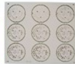
Single-layer aluminium-base PCB
