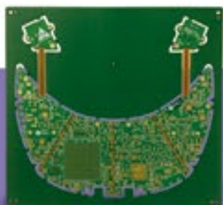
14-layer HDI rigid flex PCB
