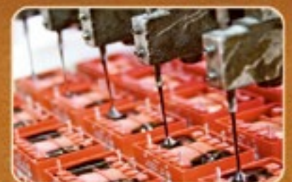
Fully automated winders with pre-twisting technology
