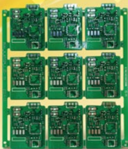
2-layer PCBs for UAV electronics • Lead-free HASL • 1mm FR4 • 1oz copper thickness
