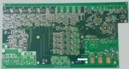
6-layer PCB with ENIG
