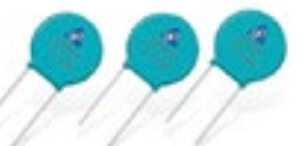
5-53D radial lead metal oxide varistors
