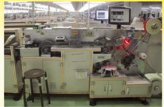
Testing, marking and tapping machines for glass-molded packages
