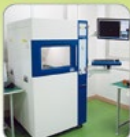
X-ray inspection and rework station for BGA devices
