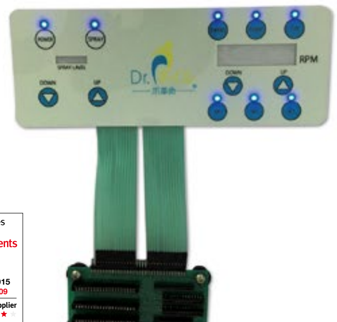
Tactile membrane switch with LED backlight and switches
