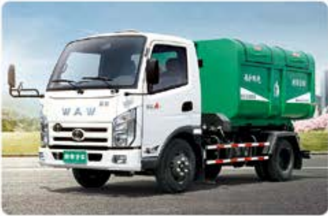
Garbage truck with detachable compartment
